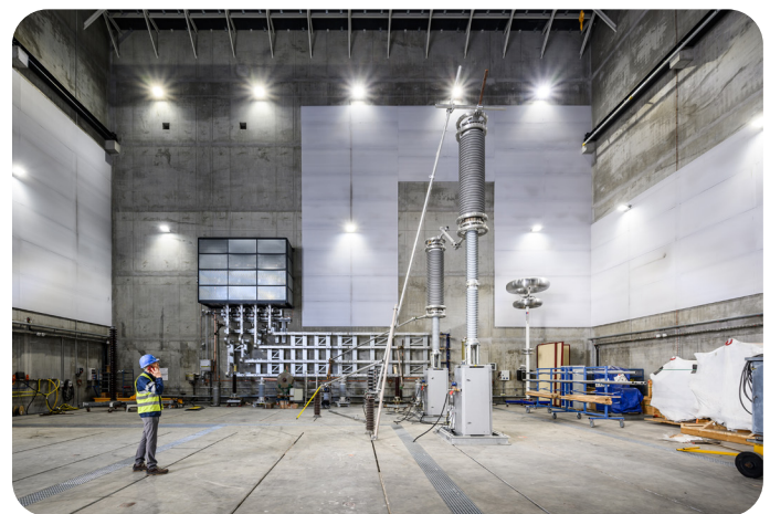
The High Power Short-Circuit test platform - 25m (L) x 25m (W) x 25m (H).
