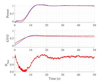
Comparison, per unit, between simulation power (blue) and generated power (red) from the hydraulic reduced scale model together with the expected (blue) and attained (red) guide vane opening (GVO) and measured head at the turbine.
