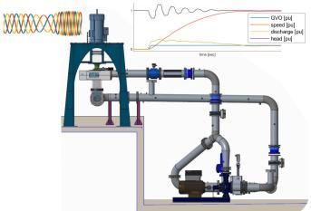
We can simulate a wide range of power conversion system layouts, including: conventional fixed speed units, DFIM variable speed, fully FED variable speed and other topologies such as Hybridised Hydro Power Plants.
