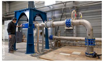
Our unique power hardware-in-the-loop hydroelectric platform to test your energy control systems.
