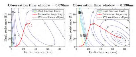
Simulations results of algorithm behavior for a fault at 80km with  $R_f$ =15 $\Omega$ . Convergence of estimated parameters at two different iteration times.
