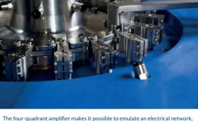
The four-quadrant amplifier makes it possible to emulate an electrical network, while the hydraulic loop permits the simulation of the network of penstocks in a real installation.
