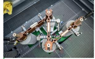
Detail of power transformers able to adapt test voltage from 6 kV up to 190 kV: connections of 6 kV secondary windings.
