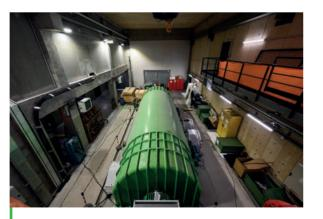
$3\,000$  MVA short circuit generator able to provide short circuit current at several frequencies, from 10 Hz up to 60 Hz.
