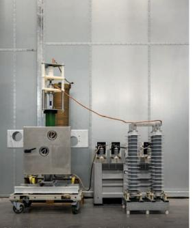
DC circuit breaker major components (left to right): vacuum interrupter with mechanical drive, inductor, small capacitor bank, four surge arresters for energy absorption
