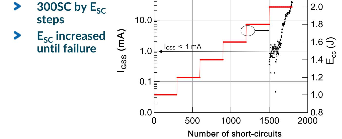
When  $V_{DS}$  is increased then the energy required to → degrade the gate oxide is decreased
